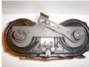
You may have to rotate the knobs till the crank cams fall into place. Notice they only turn in one direction.
