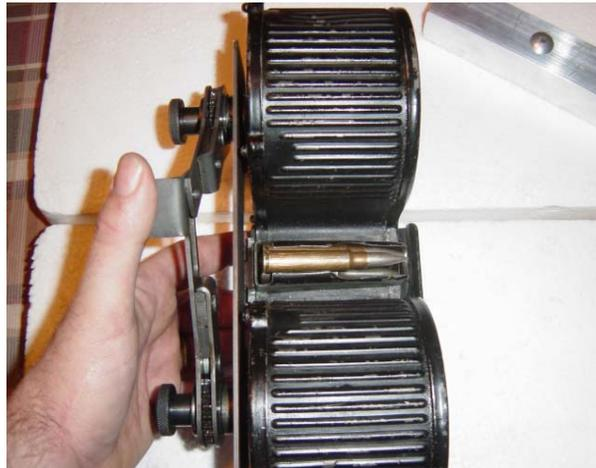
Applying pressure with your thumb you can now start inserting ammunition. When you reach the bottom of the stroke flip your thumb under the pad and push up the ratchet mechanism to reset and start installing more ammunition. Repeat till full.
