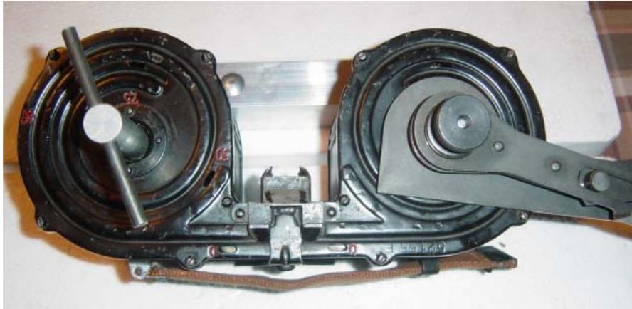
Turn the key counter clockwise and the winder clockwise to arrange the followers.
